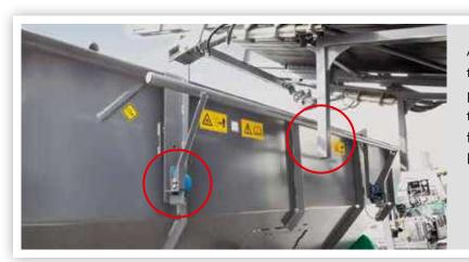
As soon as pressure is applied to the contact bar, the collision protection system ensures that the paver following the material feeder comes to an immediate halt.
