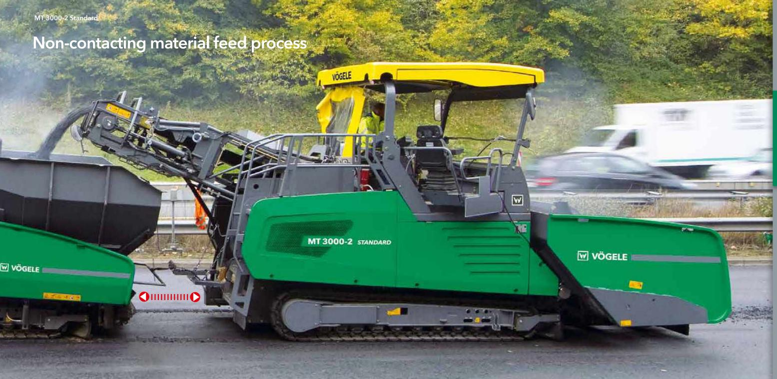
The non-contacting transfer of material is one of the key criteria for high paving quality. Decoupling the feeding from the paving process prevents the transmission of jolts from the feed vehicle to the paver when docking.
