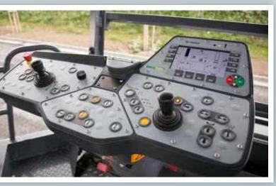
The ErgoPlus operating system comprises a well organized operator platform, the feeder operator's console with its modular design and ergonomic driver seats. This design puts the machine operator at the heart of things, guaranteeing comfort, safety and a good overview of the job site at all times.
