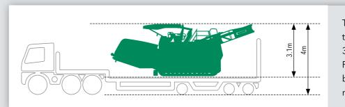
Thanks to its low transport height of 3.1m, the VÖGELE PowerFeeder can be transported on a normal low-bed trailer.
