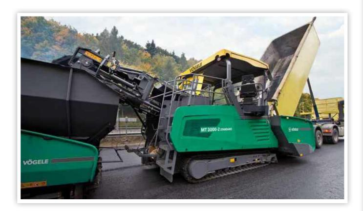
**Extremely level and durable** pavements are not a matter of chance, but are the result of clearly defined quality factors. Every interruption, e.g. because the supply of material has run out, every jolt due to the lorry docking on to the paver and any segregation of the mix is immediately evident in the quality of the built road.
